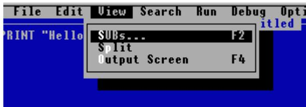
**SUBs** - Shows the list of current subroutines and functions (see *Subroutines and Functions*)
