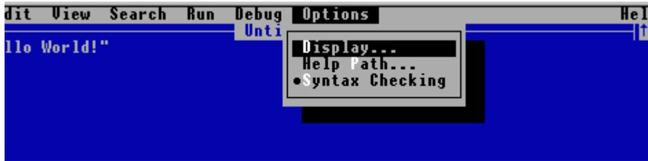
**Display** - Enables you to change display colors, the number of spaces to use for tabs, and whether or not scroll bars are visible
